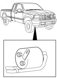
TorqShift-equipped vehicles which do not have the externally mounted filter will have the transmission fluid filter located inside the transmission bottom pan. Refer to the *scheduled maintenance information* for service intervals for automatic transmission fluid and each transmission filter type. See your authorized dealer for replacement.
